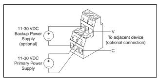
Figure 6. FP-3000 Power Connector Pinout
